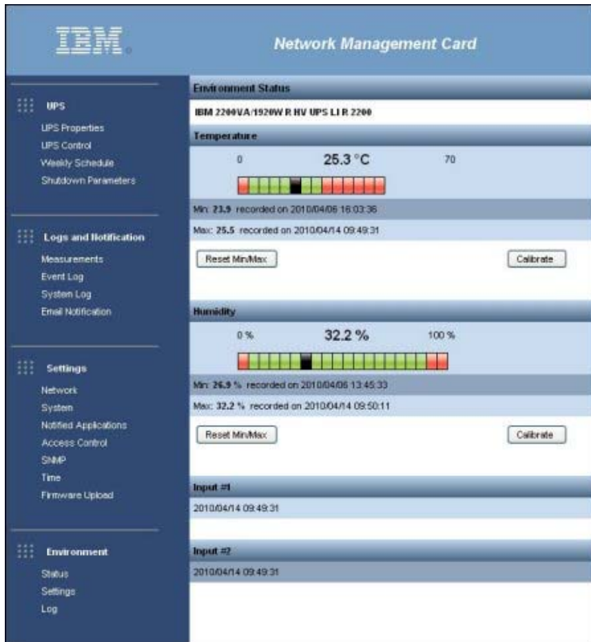
Figure 12. Environmental Monitoring Probe data as viewed from the Network Management Card web interface
